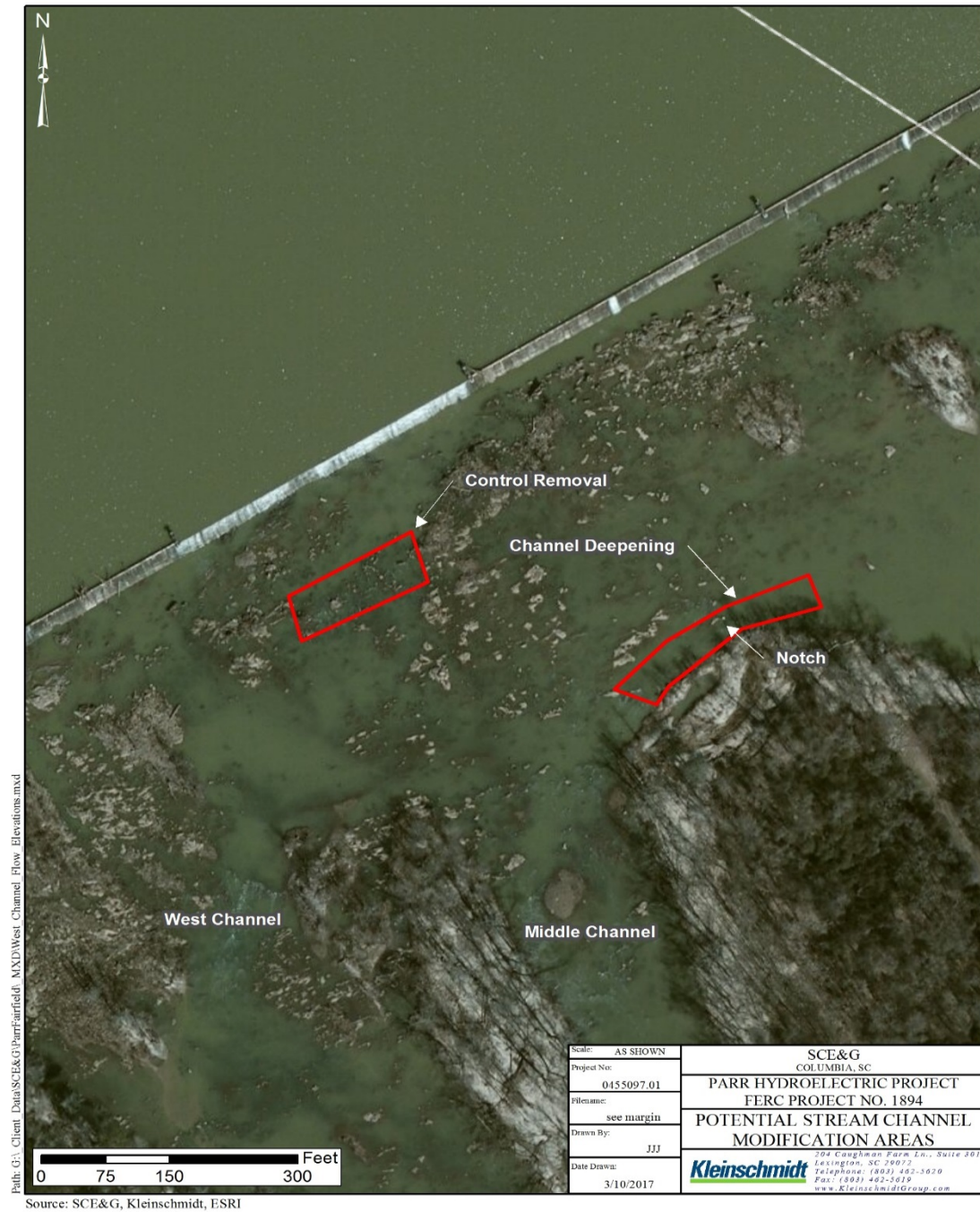
FIGURE 5-1 POTENTIAL AREAS FOR CHANNEL MODIFICATION
